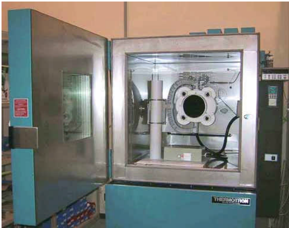
Figure 3 Thermal test chamber used to validate operational performance from -40\text{C} to 60\text{C} ( -40\text{F} to 140\text{F} ). Note the window in the chamber door permits optical xmit/rev testing in-situ.
