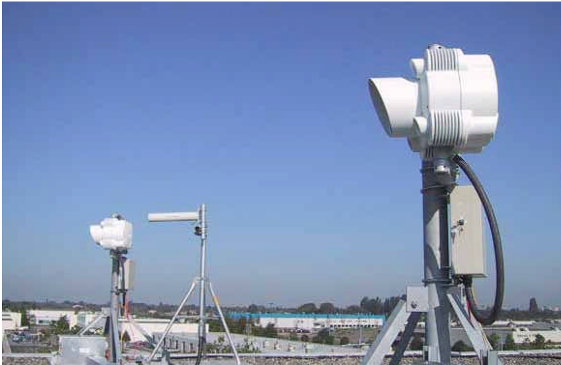
Figure 8. Two terminals being tested over the 450 meter test range from the fSONA rooftop
