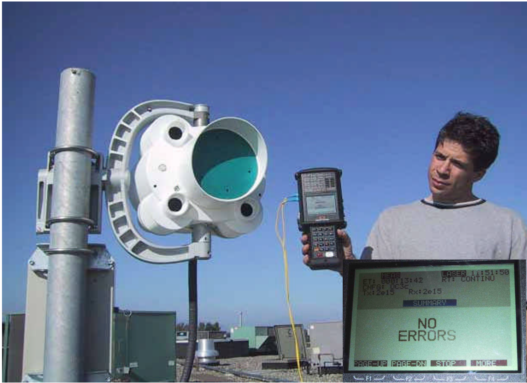
Figure 12 Error-free performance on 450 meter test range in sunny scintillation testing.
