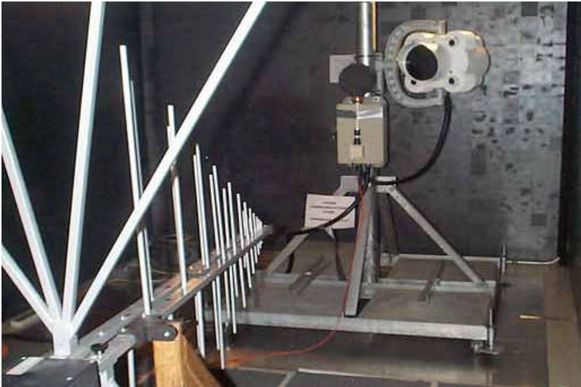
Figure 2. Extensive electromagnetic emissions and immunity testing was performed to certify the SONAbeam™ for international deployment
